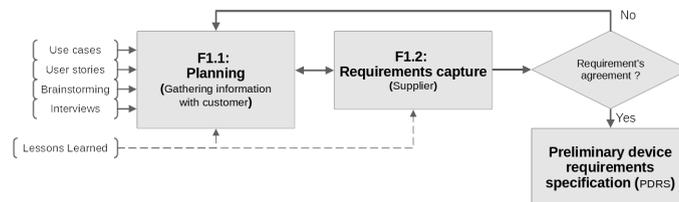
**Fig. 3.** Tasks to be completed in order to obtain a PDRS.
